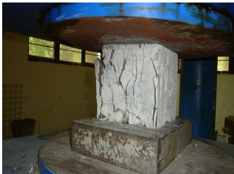
Plate 2. Cube under Compression Testing Machine
