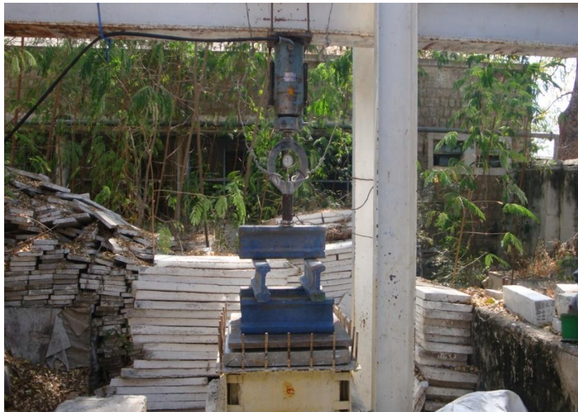
Plate 1. Slab Testing Arrangement
